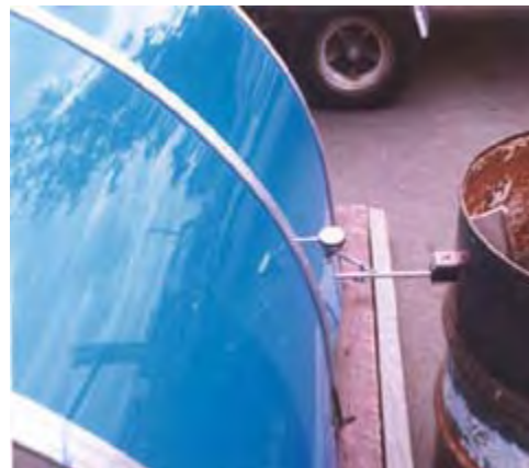
Dial Gauge for Horizontal Deflection
